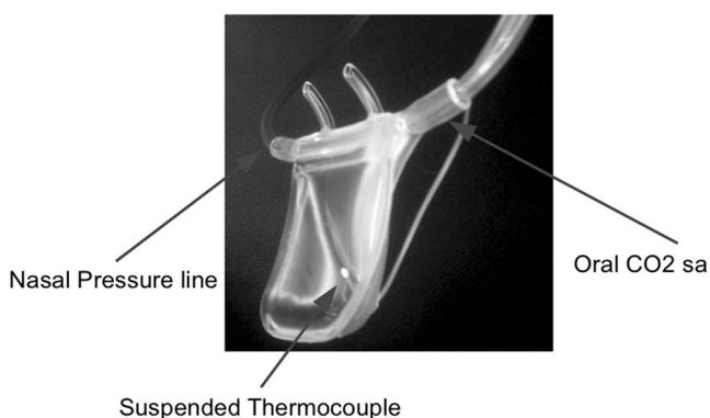
**Fig. 1** Equipment to record mouth breathing (Courtesy of Oscar Carrillo). Legend “Oral breathing is determined by a thermocouple fixed on a scoop that allows collecting flow coming from mouth breathing. The system allows to monitor nasal pressure and end tidal CO<sub>2</sub>. The system was validated using measurement of end-tidal CO<sub>2</sub> collected directly at the mouth and comparing the mouth end tidal CO<sub>2</sub> signal to the thermocouple signal [31]”
